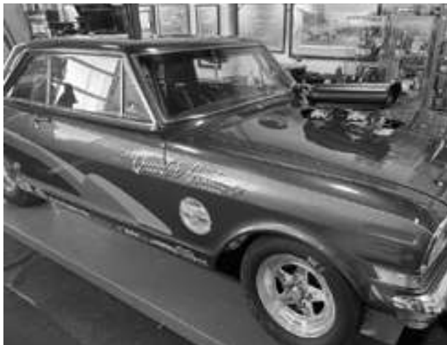
1963 Pontiac Acadian 355 , forged Eagle crank, rods, and piston's. Solid roller camshaft, roller rockers, 2.02 aluminum cylinder heads. Polished 6-71 blower, AED blower carburetors, blower scoop with K&N filters. Full exhaust. Fibreglass hood. AFCO double adjustable front shocks with delulum bushings/bearings suspension New Strange axles, and aluminum 4:57 center section. Strange disc brakes all the way around. Headlight's, signal lights, high output alternator, parking brake, street legal. Full cage. Set up for 3 speed or power glide with air shifters and controller with oil cooler. Kirkey 18" aluminum seats. Completely new electrical and fuel system. Huge aluminum radiator with electric fan. This car has been completely upgraded/renewed and built for drag and drive events....or just going to A&W. Tom Nolan $60,000 1-403-350-7873 m2
