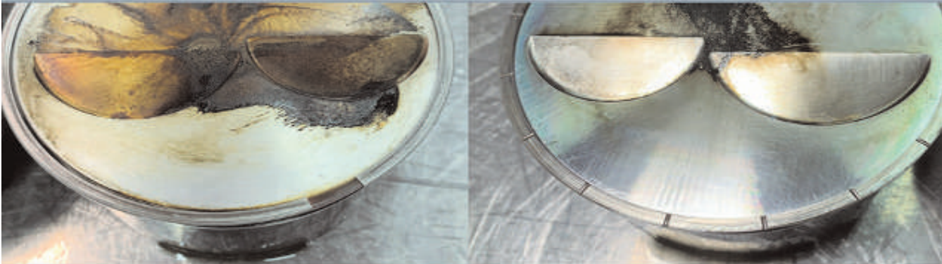
CONVENTIONAL TOP RING VS GAS PORTED TOP RING
