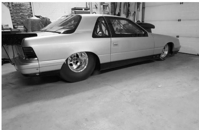
1992 LeBaron 750 cert. mild steel, steel roof, quarters, everything else fiberglass. 565 BB Chev. Dart block. Pro One Heads, JW 2 speed transmission. New front and rear tires. $29,500 Call 403-830-1256 for more info. Calgary, AB. M1
