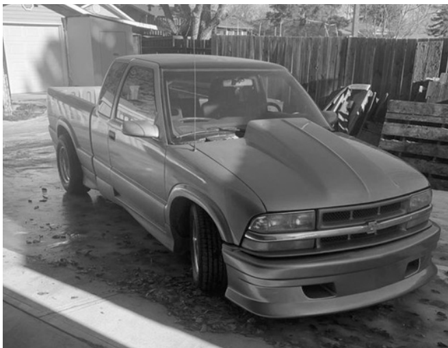
2001 s10 street truck. Built 350, rpm heads, 1552 polished blower, blower cam, msd pro billet dist, coil, 6btm ignition, boost retard in cabin adjust, ceramic long tubes, polished alt., full painless harness Built th350, B&m pan, forward shift manual valve body, line lok, trans brake
